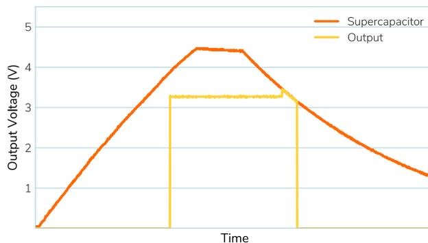
Charge/Discharge @ 3.3V Output with Battery Backup
